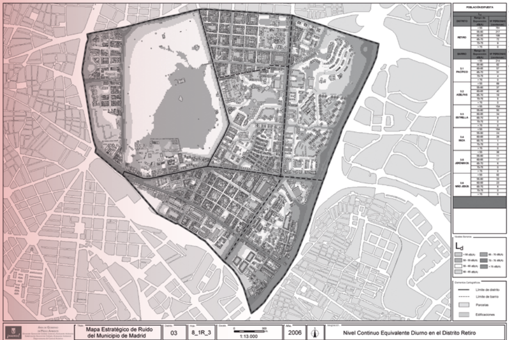
Fig. 1 Example of conventional acoustic mapping. Strategic noise map. Continuous equivalent daytime noise level. Retiro District. Madrid. Source: Madrid City Council.
